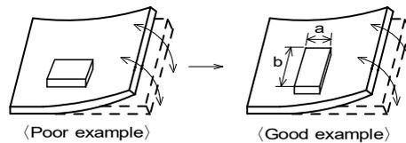
(2) Components location on PCB separation
